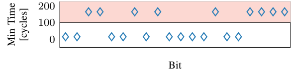
Figure 17: Flush+Fault: 20 RSA key bits (C906). ‘1’ bits are above, ‘0’ bits below 100 cycles.
